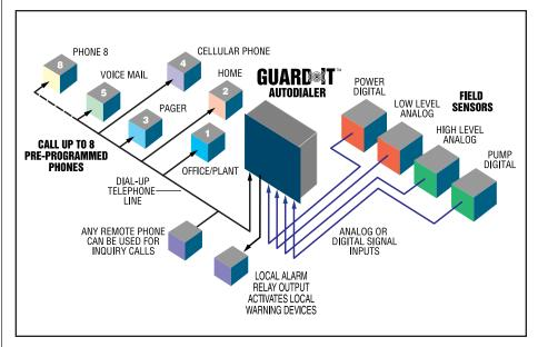
Guard-It Systems have four inputs which can be configured for either analog or digital sensing. The system can call up to eight preprogrammed phone numbers over the standard dial-up telephone and cellular networks.
